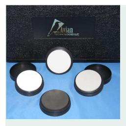
Gray scale standards are essential for establishing the photometric linearity of a reflectance spectrometer.
