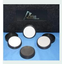
Gray scale standards are essential for establishing the photometric linearity of a reflectance spectrometer.
