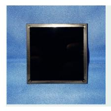
Avian Technologies' Low-Reflectance Specular Standard consists of a 2" square of highly polished Schott UG-11 glass backed by a low reflectance diffuse material to absorb any transmitted radiation, all encased in a black Delrin holder. The standard may be used to characterize systems where a standard first surface mirror would be too reflective.
