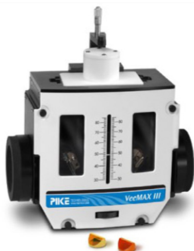
Electrochemical Cell assembly for VeeMAX III.
