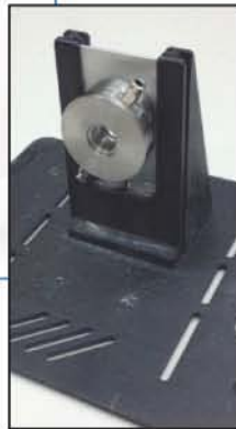
Dynamic Sealed Liquid Cell SL-15 (above) and mounted in a cell holder (right) on a universal baseplate.
