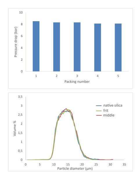
A DAC column with 5 cm internal diameter was used. 5 packings/unpackings to 100 bars were made with the same silica slurry.
