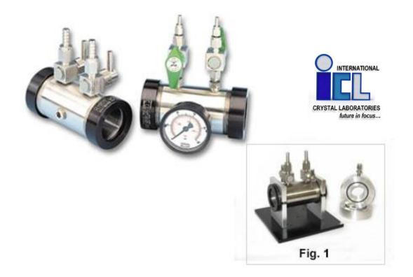
The G-2SS stainless steel gas cell is useful for qualitative analysis of pure gases and mixtures where one or more of the constituent gases are present in concentrations of at least 5 percent. It can be used in situations that make use of a glass cell impractical, such as applications involving high pressure or gases that etch a glass cell body.
