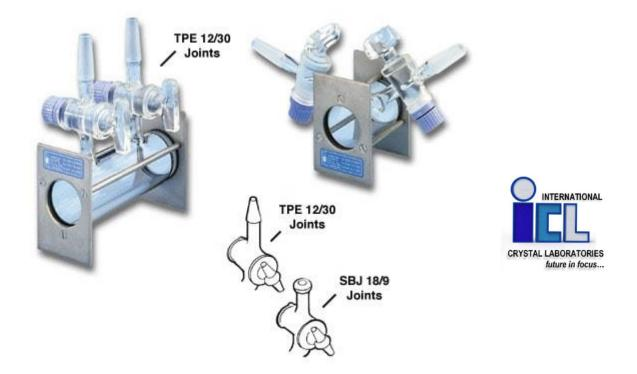
The G-2 Gas Cell is for analysis of pure gases or gas mixtures in which component gases are present at concentrations of 5 percent or more. The G-2 Gas Cell has a fixed pathlength of either 5cm or 10cm. The windows of the cell are easy to remove for cleaning, making the G-2 ideal for working with wet or reactive gases that have a tendency to fog or attack the window material.
